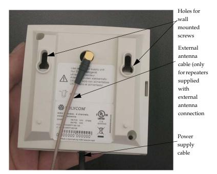
**Figure 6-2** Connect Power to the Bottom of the Repeater and External Antenna Cable to the Rear of the Repeater
