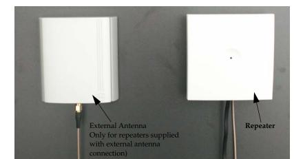
Figure 6-3 Repeater and External Antenna Installed on the Wall
