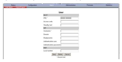
The data configured for each handset can be split into two categories. DECT data which is necessary for the correct handling of the DECT protocol stack. SIP data which is necessary for the handling of a SIP user agent.
