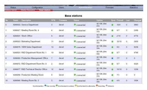
Figure 15-41 Sync States of Base Station - Colour Description
