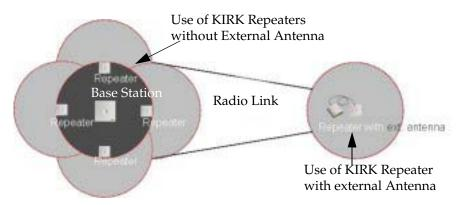
The distance from the repeaters without external antenna to the base station must correspond to a RSSI loss of maximum 25dB.
