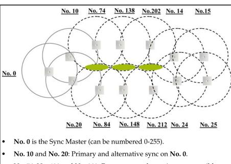
Figure 3-8 Synchronization Chain With Repeaters
